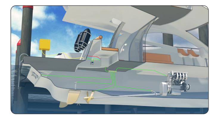
There are many different compositions of wires and lugs used by Marine electricians. Some of these materials are not effective for use in a bonding system and as such the galvanic current is not carried. Additionally of there is a break in the bonding system such as a faulty connection or damaged wire it can also leave the vessel inadequately protected.
