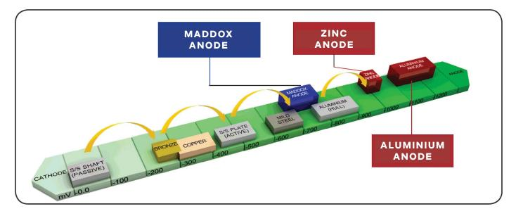
The Galvanic Series of Metals can be used to determine the tendency of a galvanic reaction and subsequent galvanic corrosion. American Boat and Yacht Council (ABYC) E-2 Cathodic Protection notes:
